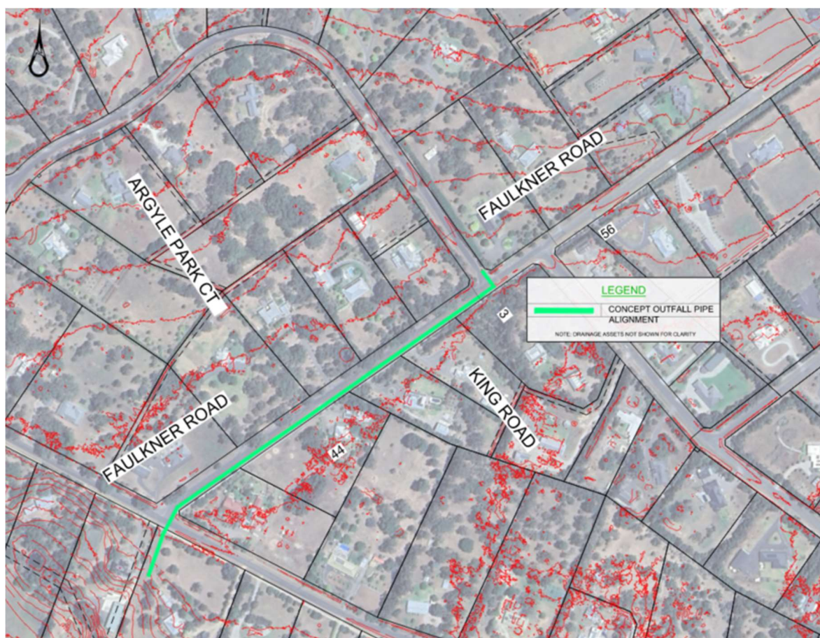
Figure 23 –Concept sketch of Option 3a Piped conveyance of flows along Faulkner Road
