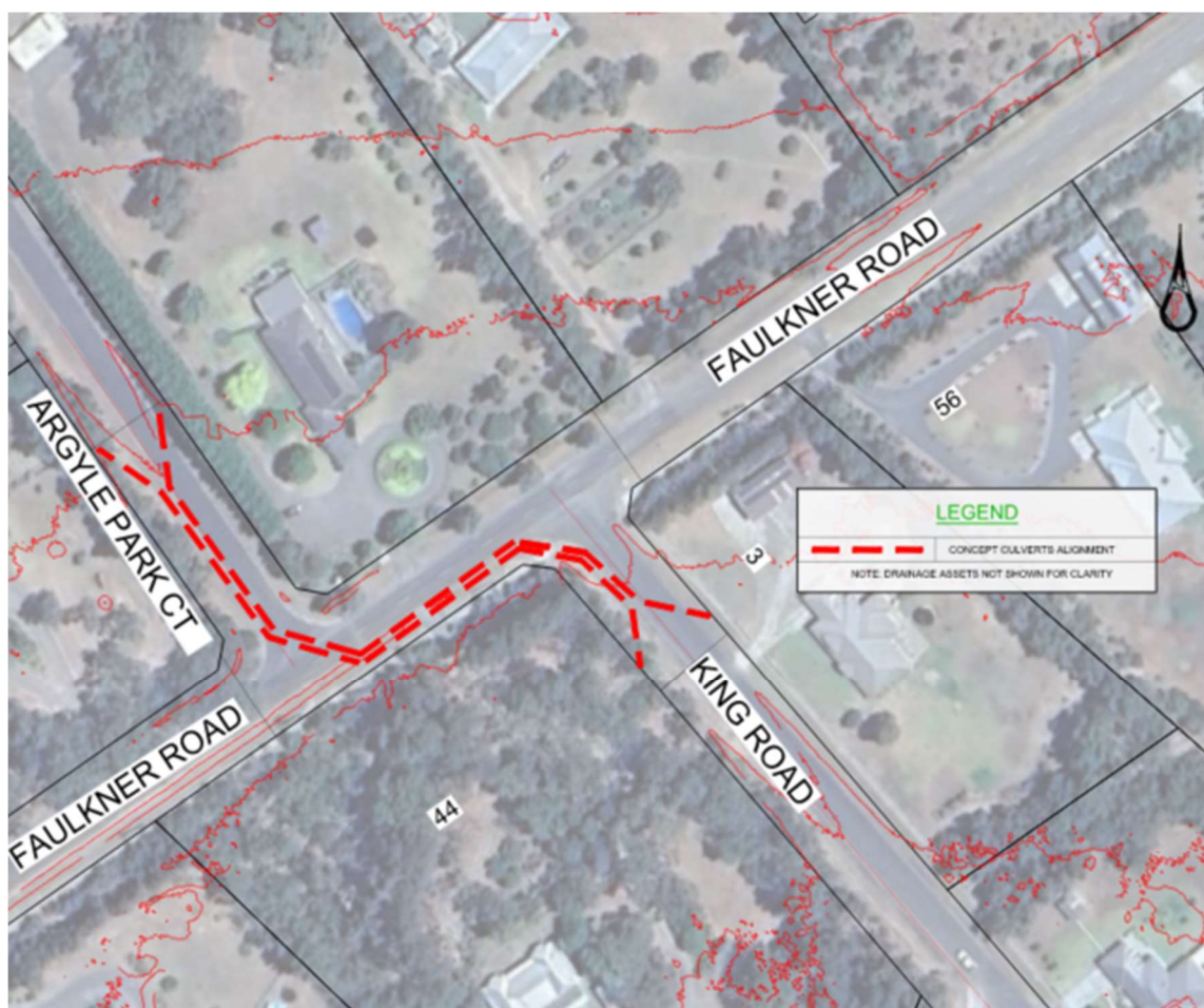
Figure 9 –Concept sketch of Option 1a piped conveyance of flows from Argyle Park Court to King Road
