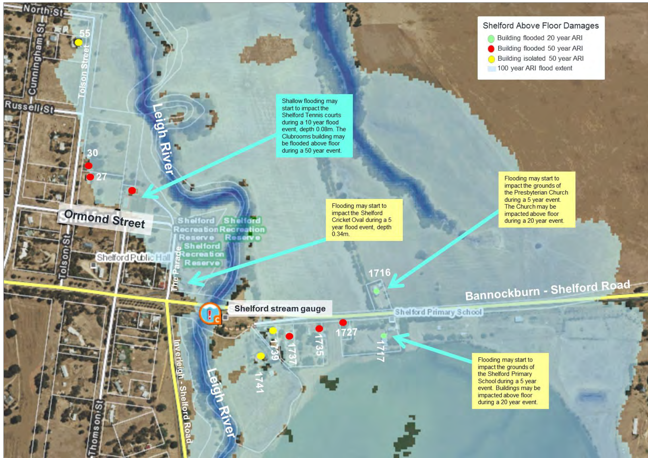
Figure 38. Shelford buildings subject to above floor flooding (source: Corangamite CMA Flood Response Guide and anecdotal observations).
