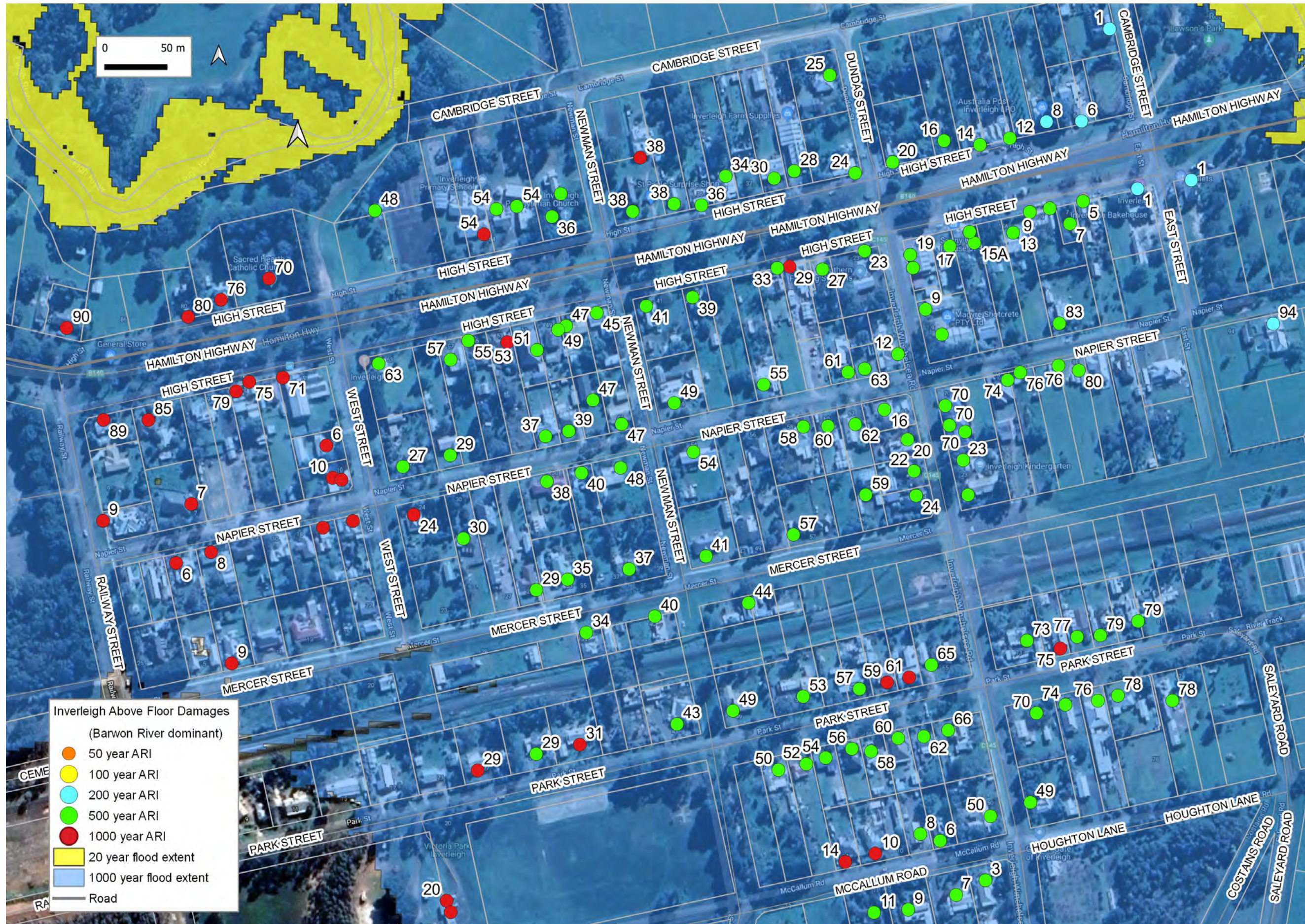
Figure 31. Inverleigh above floor damages over a range of design flood events for a Barwon River dominant flood (Water Technology 2018).
