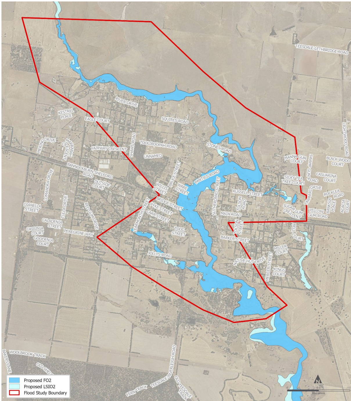
Figure 1: Teesdale amendment overlay areas showing the extents of the proposed FO2 and LSI02. Note the overlay extents that are outside the study area remain unchanged.
