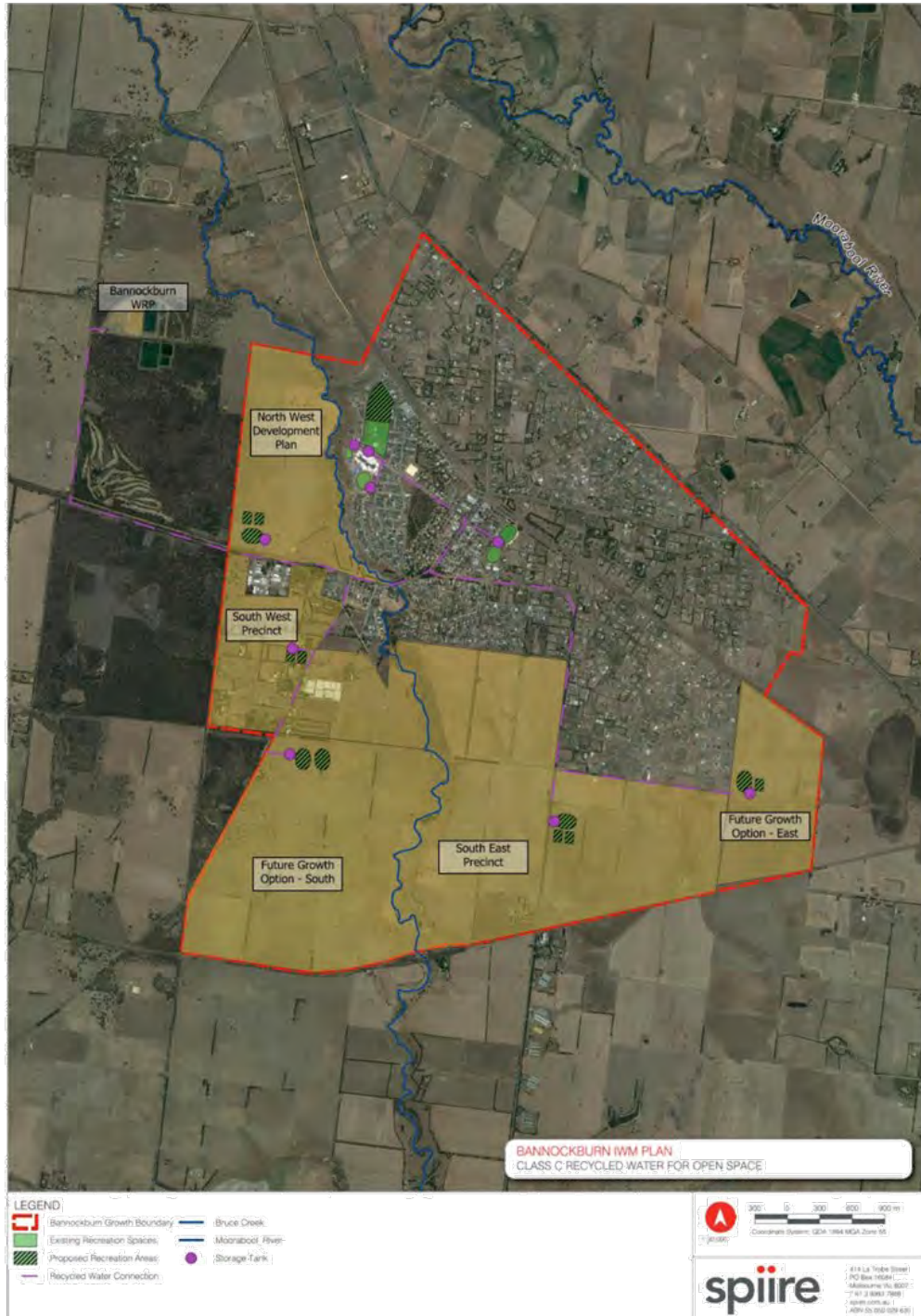
Figure 25: Concept layout of the Class C recycled water to open space irrigation option
