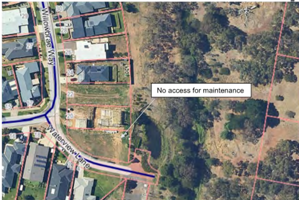
Figure 19: A stormwater detention basin that has no access track for maintenance activities
